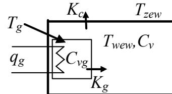
$$\begin{cases} C_{vg} \dot{T}_{gp}(t) = q_g(t) - K_g(T_g(t) - T_{wew}(t)) \\ C_{vw} \dot{T}_{wew}(t) = K_g(T_g(t) - T_{wew}(t)) - K_c(T_{wew}(t) - T_{zew}(t)) \end{cases}$$
