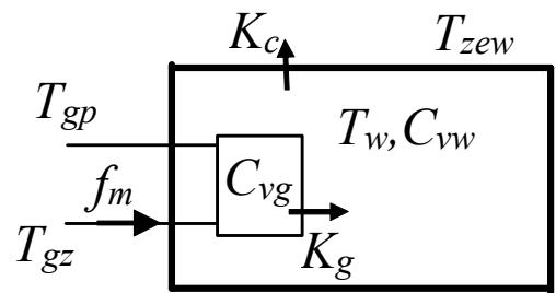
$$\begin{cases} C_{vg} \dot{T}_{gp}(t) = c_{pw} f_m(t)(T_{gz}(t) - T_{gp}(t)) - K_g(T_{gp}(t) - T_{wew}(t)) \\ C_{vw} \dot{T}_{wew}(t) = K_g(T_{gp}(t) - T_{wew}(t)) - K_c(T_{wew}(t) - T_{zew}(t)) \end{cases}$$
