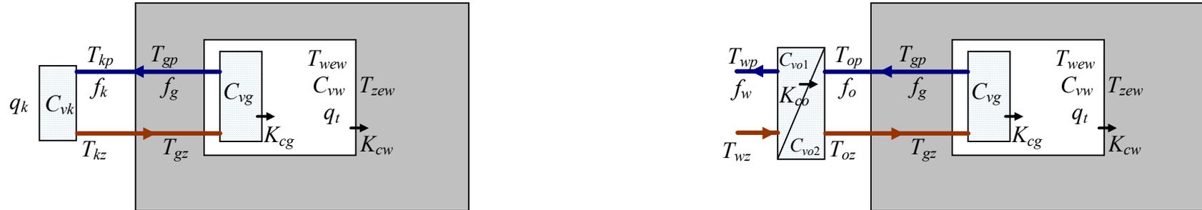
$$\begin{cases} C_{vw} \dot{T}_{wew} = K_{cg} (T_{gp} - T_{wew}) - K_{cw} (T_{wew} - T_{zew}) + q_t \\ C_{vg} \dot{T}_{gp} = c_{pw} f_{mg} (T_{gz} - T_{gp}) - K_{cg} (T_{gp} - T_{wew}) \end{cases}$$
