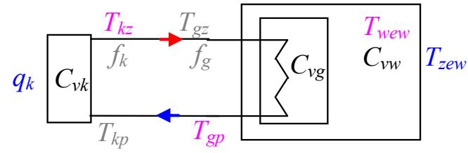
$$\begin{cases} C_{vw} \dot{T}_{wew} = K_{cg} (T_{gp} - T_{wew}) - K_{cw} (T_{wew} - T_{zew}) \\ C_{vg} \dot{T}_{gp} = c_{pw} \rho_w f_g (T_{gz} - T_{gp}) - K_{cg} (T_{gp} - T_{wew}) \\ C_{vk} \dot{T}_{kz} = q_k - c_{pw} \rho_w f_k (T_{kz} - T_{kp}) \end{cases}$$
