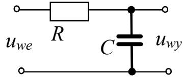
$$\begin{aligned} Z_1 &= R \\ Z_2 &= 1/sC \end{aligned}$$
