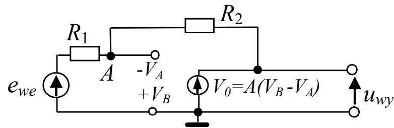
$$\begin{cases} \frac{V_A - e_{we}}{R_1} = \frac{V_0 - V_A}{R_2} \\ u_{wy} = V_0 = A(V_B - V_A) = -AV_A \end{cases}$$
