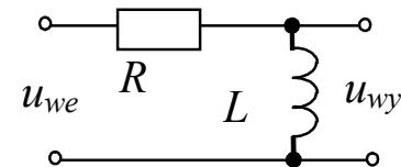
$$\begin{aligned} Z_1 &= R \\ Z_2 &= sL \end{aligned}$$
