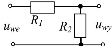
$$u_{wy}(s) = \left( \frac{R_2}{R_1 + R_2} \right) u_{we}(s)$$
