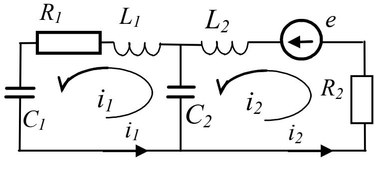
$$\begin{cases} e = sL_2 i_2 + R_2 i_2(s) + \frac{i_2 - i_1}{sC_2} \\ 0 = sL_1 i_1 + R_1 i_1 + \frac{i_1}{sC_1} + \frac{i_1 - i_2}{sC_2} \end{cases} \quad \text{rząd?}$$
